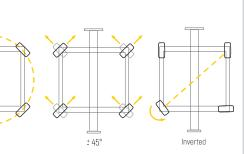
Polar: The unit rotates 360° on its own axis. ±45°: Movement in both diagonal directions. Inverted: Movement using the 2 back wheels.
