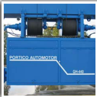
SOUNDPROOF POWER UNIT
